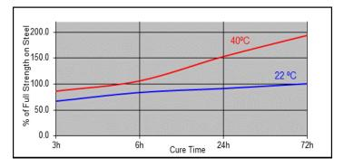
The table below shows breakloose torque developed with time on 3/8inch NPT steel pipe tees and plugs, pretorqued to 238 in-lb and tested according to ASTM D6396.
