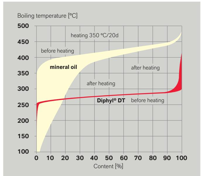
Thermal stability acc. to DIN 51528, simulated distillation GC with Diphyl® DT and mineral oil
