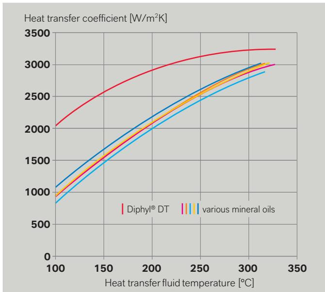
Heat transfer coefficient of Diphyl® DT compared with various mineral oils
